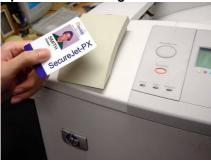
SecureJet Auth-PX is a sophisticated badge reader directly connected to the hp LaserJet MFP motherboard, combined with a software running inside the printer.
